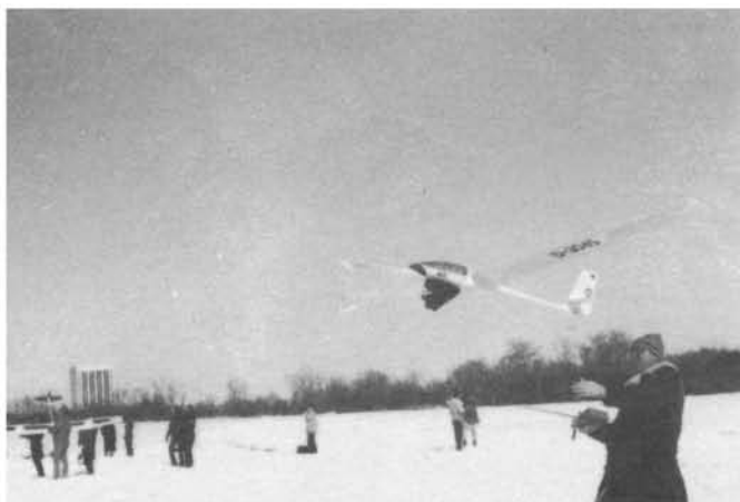
Jack Hiner, sans gloves, launches his SB-10, built from Carrera kit described in April MA column. This version has a 3200-mm wing span.
